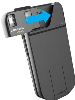
3. Verify that the top hook on the optics housing is fully engaged with the slot in the top of the OtterBox uniVERSE case. You may need to use your thumb to push it into place.
